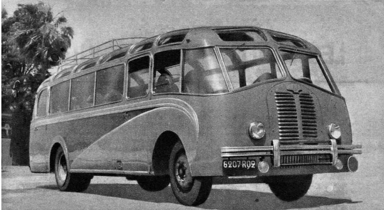
CAR CURRUS DE GRAND LUXE, 30 PLACES, CHASSIS DELAHAYE 163 L, MOT. DIESEL 80 CH. A L'AV.
