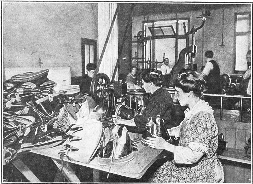
LE PERÇAGE DES TROUS DANS LE TURBAN DE LA COIFFE
