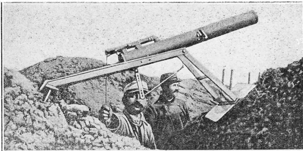
LANCE-BOMBES FRANÇAIS MONTÉ SUR UN CHASSIS PERMETTANT LE POINTAGE
